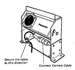
2. Change the direction of the camera fixing plate as follows.
