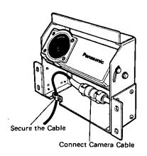
Secure the camera onto the rear-end of the roof using 4 bolts (prepared locally (6mmφ bolt)).
