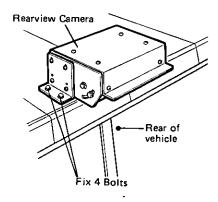
Note: Secure the camera so that the camera positions in parallel with the rear-end line of vehicle.
