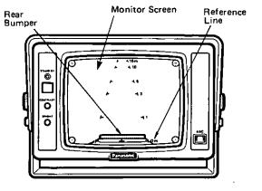
4. Adjust the camera tile by loosing 4 hex bolts so that the rear bumper positions on the reference line of the distance chart on the monitor screen.
