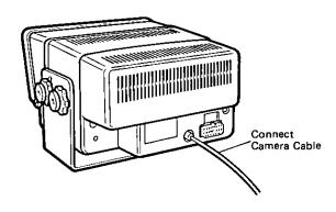
Connect the supplied remote cable for monitor to the power and remote connector on the rear of the monitor.
