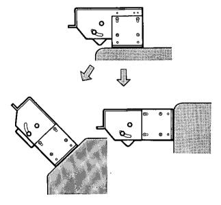
3. Secure the camera onto the rear panel of the vehicle.
