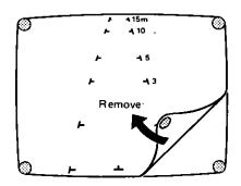
Clean the monitor screen and put the distance seal onto the monitor screen after removing the reverse paper on the glues on the 4 corners of the seal.
