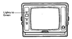
Whenever changing the gear shift to the reverse position, the Mode Indicator (12) LED turns into amber (ON mode) and the rearview picture can automatically be seen on the monitor screen in few seconds.
