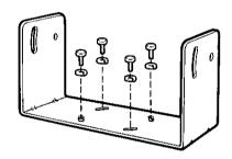
3. Secure the monitor onto the monitor fixing plate using supplied 4 monitor fixing screws and adjust the tilt of the monitor.
